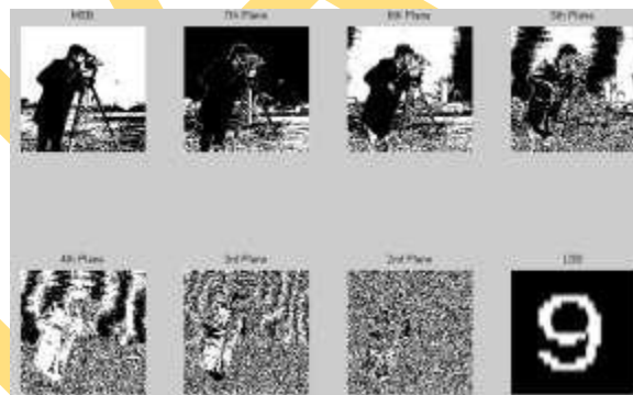
Fig.9: Least Significant Bit is replaced with message
